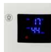
LCD screen with relative humidity and ambient temperature indicator.
